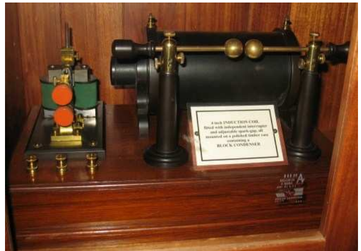
4 inch Induction coil fitted with an independent interrupter and adjustable spark coil
